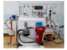
Fig. 1. General view of the experimental setup for determining the efficiency of the acoustic-magnetic water treatment device
